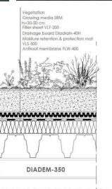
Vegetitilan Growing media SRM In-93-33 cm Mineral subditate MS-h25-40 cm Filler sheet VLF-200 Drainage board Diadrain-60H Mobilure refension & protection me VLS-600 antirool membrane FLW-400
