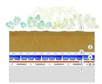
1. Vegetation, 2. Vegetation substrate SEM, 3. Geotextile filter VLF-150, 4. Drainage board **DiaDrain-25H**, 5. Protection fleece VLU-300, 6. Root protection layer FLW-400, 7. Roof construction
